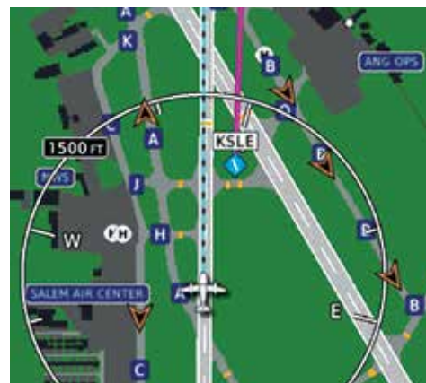
TerminalTraffic™ Feature is available with SafeTaxi® to enhance the pilot's traffic situational awareness in the airport environment by displaying surface targets for ADS-B-equipped taxiing aircraft and ground vehicles on the airport diagram.
