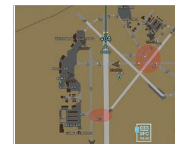
Optional SafeTaxi diagrams with georeferencing capability help you navigate on unfamiliar airports. With an optional GDL 52 series receiver, TerminalTraffic technology displays ADS-B equipped surface targets right on these diagrams.
