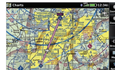
IFR Enroute and VFR Sectional charts for the U.S. feature georeferencing capability – with an overlaid aircraft symbol indicating your current position.
