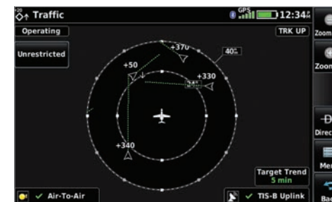
With ADS-B "In" from a compatible receiver (sold separately), the aera 660 and aera 760 can display traffic enhanced with Garmin TargetTrend™ technology, which shows target trajectories relative to your aircraft.
