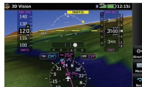
Database-driven 3D Vision display offers a simulated terrain view in context with your aircraft. You can rotate the 3-D view completely around the aircraft for easy scanning from various "camera ship" perspectives.
